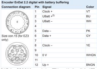
2) UBatt+ = DC 3.6 V for encoder type EBI in combination with the AES option of STOBER-drive controllers
