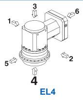
**IMPORTANT:** Mounting PHKX in either vertical mounting position (EL3 or EL4) must be specified when ordering.
