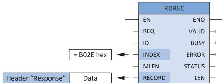
Fig. 9: RDREC system function block: Input and output parameters
