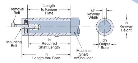
STOBER reducers with a hollow output can be mounted to the equipment shaft from either side. Tolerances for the hollow bore are shown in Table 1. Be sure to tolerance the equipment shaft to fit accordingly.
