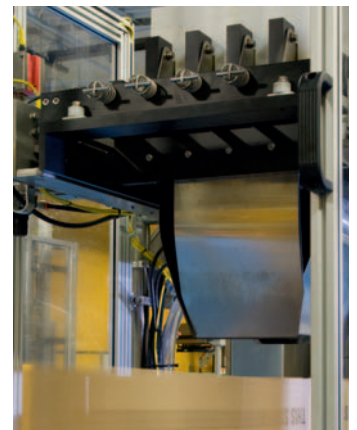
High-speed filling movements are precisely coordinated with each other using the AS6 Automation Control Suite
