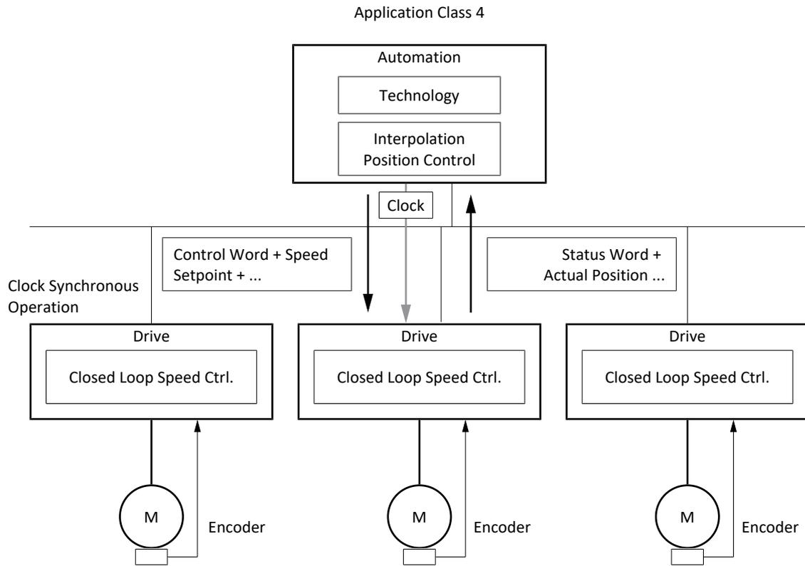
Fig. 33: PROFIdrive: Application class 4 (source: PROFIdrive profile)
