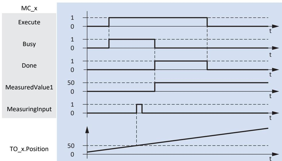
Fig. 44: Sequence of the measuring input function
