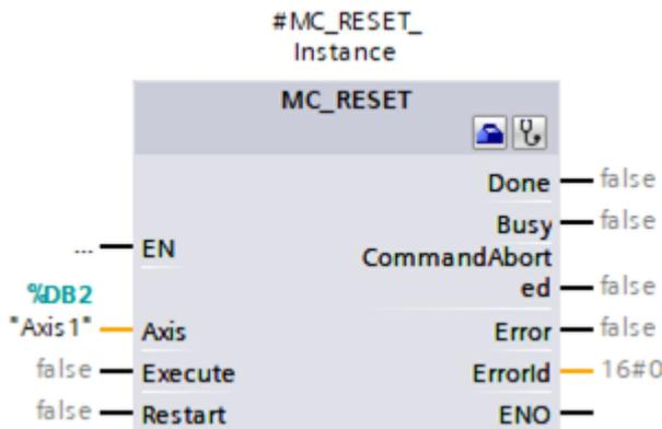
Fig. 16: PLCopen block MC\_RESET
