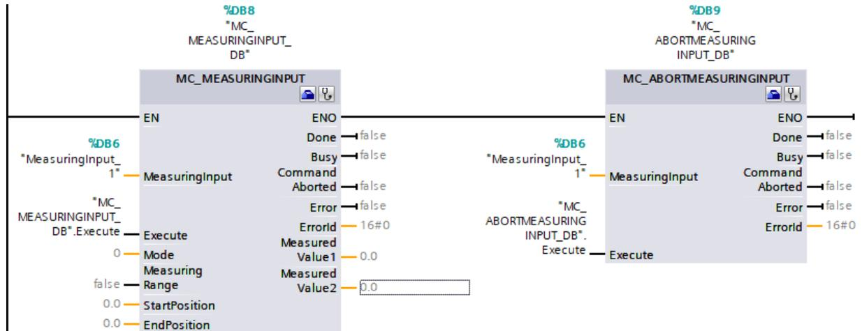
Fig. 9: PLCOpen blocks MC\_MEASURINGINPUT and MC\_ABORTMEASURINGINPUT
