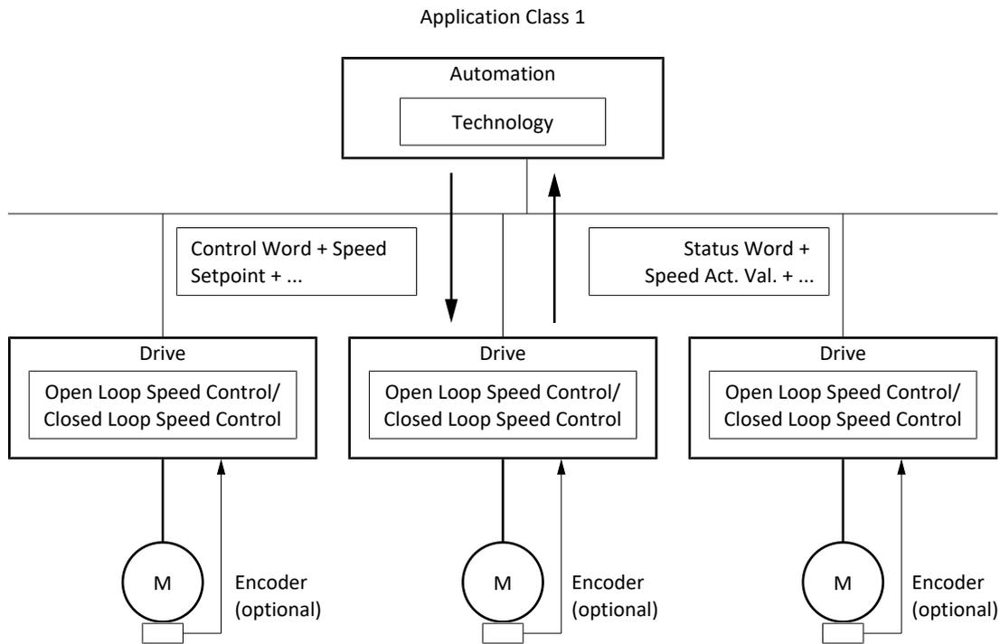
Fig. 26: PROFIdrive: Application class 1 (source: PROFIdrive profile)
