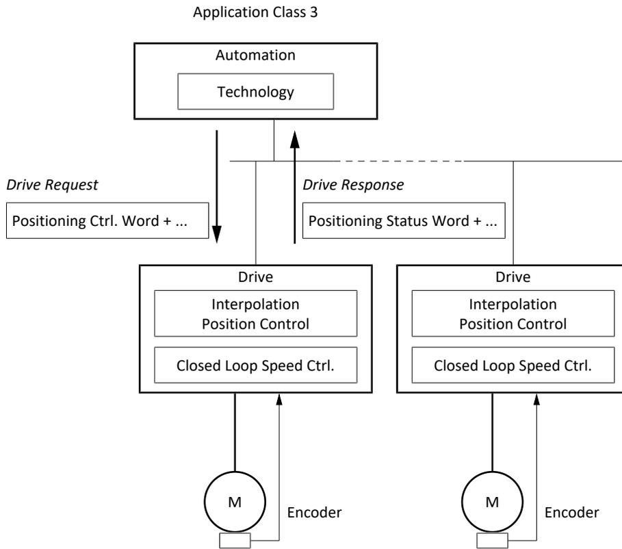
Fig. 31: PROFIdrive: Application class 3 (source: PROFIdrive profile)
