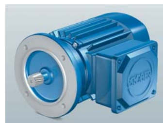
MGS Systemmotor AC asynchronous motor Motor power: 0.12 – 45 kW Optional: Brake, forced cooling fan, incremental encoder or multturn absolute encoder Additional design versions for special area applications: Ex, underwater, hygiene, food
