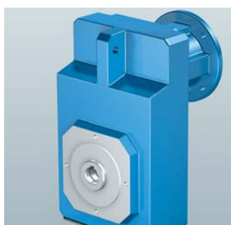
MGS F Shaft-Mounted Helical Gear Unit 5 sizes: F1 – F6 Rated torque: 45 – 1,100 Nm Gear ratio range: 4 – 600 Backlash standard: \leq 10 - 11 arcmin Reduced class II: \leq 5 - 8 arcmin Extremely flat gear housing and great shaft-centre distance
