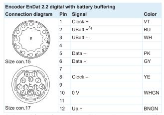
3) UBatt+ = DC 3.6 V for encoder type EBI in combination with the AES option of STOBER-drive controllers
