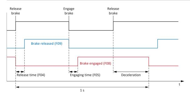
Fig. 75: Minimum time between two release processes for the brake
