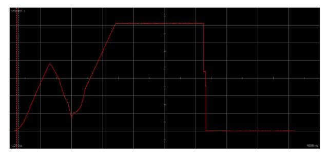
Fig. 70: Scope – Motor reaches saturation with tracking (B59)
