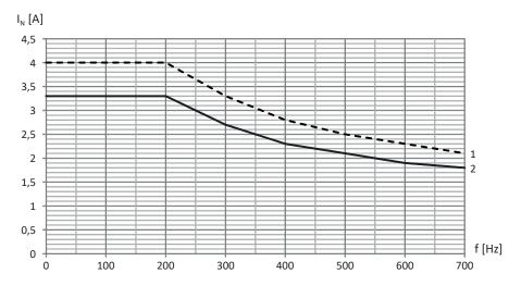
Fig. 22: Derating the nominal current depending on the clock frequency, TEP3720-0ES41
