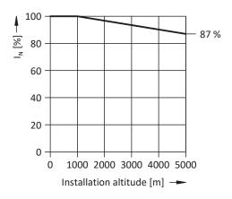
Fig. 20: Derating the nominal current depending on installation elevation  $% \left( 1\right) =\left( 1\right) \left( 1\right)$
