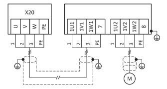
Fig. 54: TEP output choke connection example
