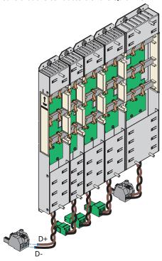
2. Place the drive controller or supply module on the bottom threaded bolt(s) of the Quick DC-Link module and properly align the device vertically with the bottom and top threaded bolts.
