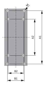
Fig. 42: TEP drilling diagram
