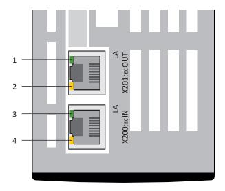
Fig. 90: LEDs for the state of the EtherCAT network connection
