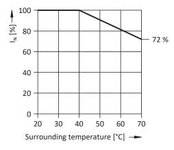
Fig. 25: Derating the nominal current based on surrounding temperature
