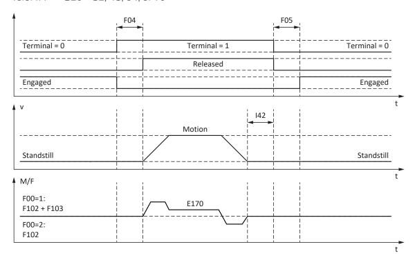
Fig. 74: Brake control for control mode B20 = 32: LM - sensorless vector control, 48: SSM-vector control incremental encoder, 64: SSM - vector control or 70: SLM - vector control
