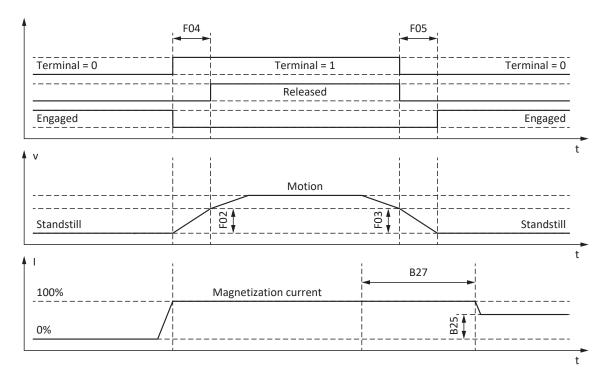
Fig. 73: Brake control for control mode B20 = 3: ASM - sensorless vector control
