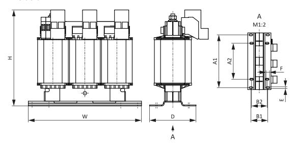
Fig. 18: TEP dimensional drawing
