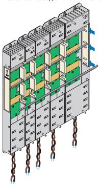
6. Fasten the copper rails with quick fastening clamps (DL6B10 to DL6B21 with two, DL6B22 with three quick fastening clamps per rail). Make certain the contact points of the copper rails do not become contaminated.
