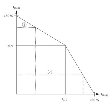
Fig. 9: Asymmetric load on double-axis controllers
