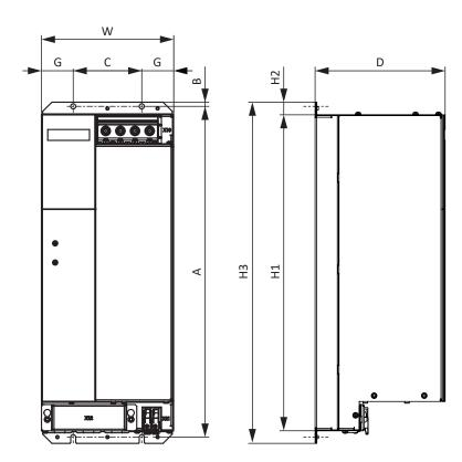
Fig. 8: PS6A44 dimensional drawing
