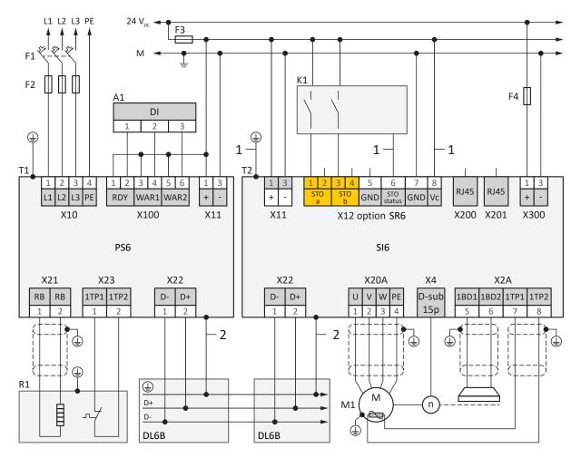
Fig. 95: Wiring example with a PS6A24 or PS6A34 supply module
