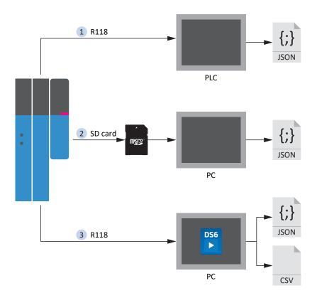
Fig. 80: Predictive Maintenance: Options for readout
