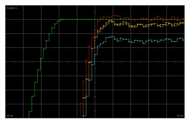
Fig. 66: Scope – Integral coefficient of the velocity controller (C32)
