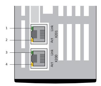
Fig. 91: LEDs for the state of the PROFINET network connection
