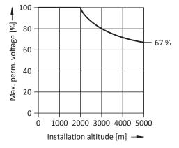
Fig. 21: Derating the voltage depending on installation elevation
