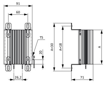
Fig. 13: KWADQU dimensional drawing with MWS306L
