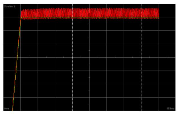
Fig. 62: Scope – Proportional coefficient of the velocity controller (C31), continuous oscillations
