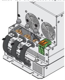
6. Reattach the cover of X22 using the two fastening screws (2.3–2.9 Nm).
