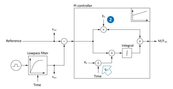
Fig. 60: Velocity controller – Proportional coefficient
