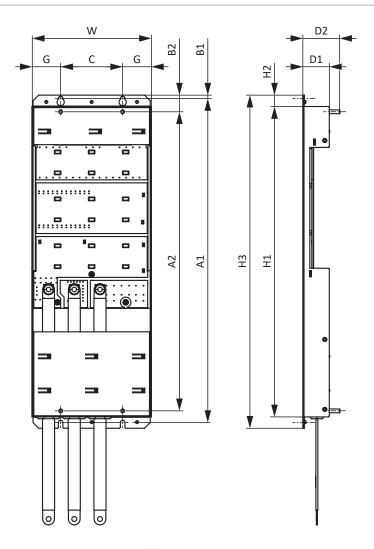
Fig. 12: DL6B22 dimensional drawing
