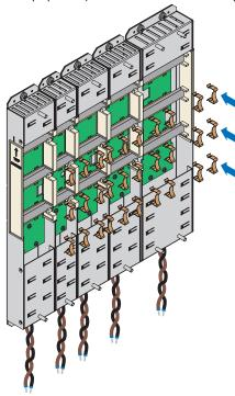
⇒ You have installed the Quick DC-Link. In the next step, build over the Quick DC-Link modules with suitable drive controllers and supply modules.
