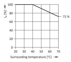
Fig. 19: Derating the nominal current based on surrounding temperature
