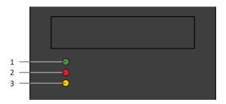
Fig. 81: Diagnostic LEDs on the front of the PS6 device
