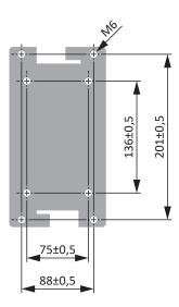
Fig. 41: Power choke drilling diagram
