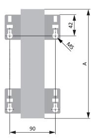
Fig. 38: KWADQU drilling diagram with MWS 310L
