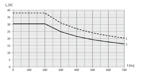
Fig. 24: Derating the nominal current depending on the clock frequency, TEP4020-0RS41
