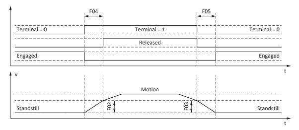
Fig. 71: Brake control for control mode B20 = 0: ASM - V/f-control or 1: ASM - V/f-slip compensated
