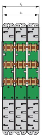
Fig. 43: Determination of the correct length of the copper rails
