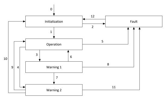
Fig. 82: PS6 device state machine
