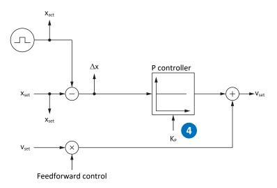
Fig. 67: Position controller - Proportional coefficient
