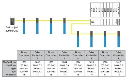
Fig. 100: Test setup of the application examples
