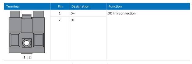
Tab. 146: X22 connection description, sizes 2 (double-axis controllers) and 3  $\,$
