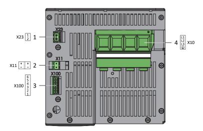
Fig. 47: PS6A44 connection overview, top of device
