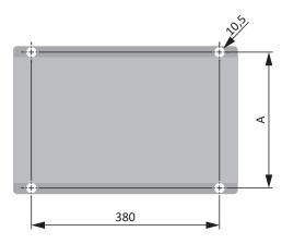
Fig. 40: FGFKQU drilling diagram
