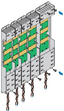
2. Insert the insulation connection pieces between the modules and insulation end section each at the left edge of the first module and at the right edge of the last module. Ensure correct alignment of the end section using the marking on the outside and the insertion aids for the copper rails on the inside.
