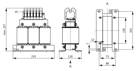
Fig. 17: Power choke dimensional drawing
