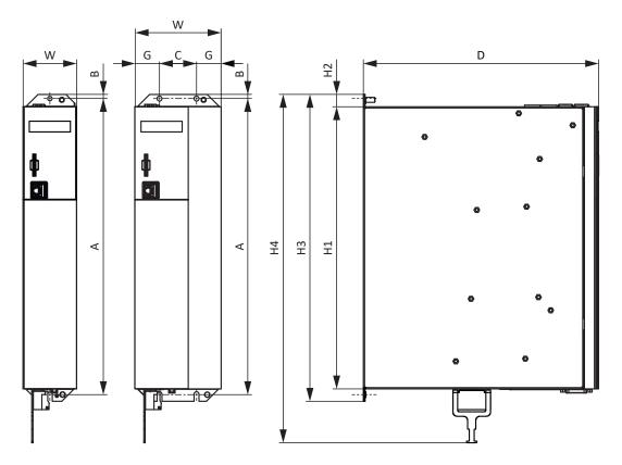
Fig. 10: SI6 dimensional drawing
