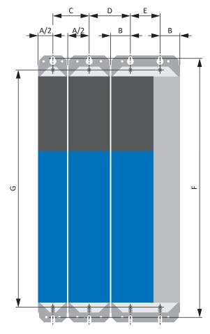
Fig. 35: Drilling diagram of DL6B10 to DL6B21
