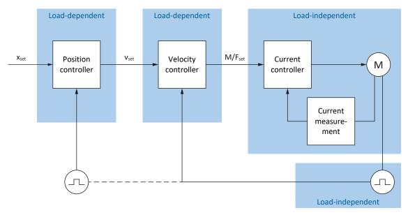
Fig. 57: Structure of the control cascade
