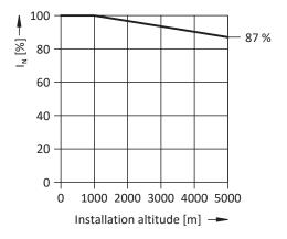
Fig. 26: Derating the nominal current depending on installation elevation
