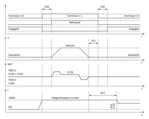
Fig. 72: Brake control for control mode B20 = 2: ASM - vector control
