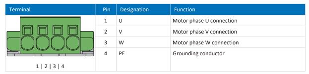
Tab. 142: X20A connection description, sizes 2 (double-axis controllers) and 3
