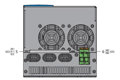
Fig. 48: PS6A44 connection overview, bottom of device
