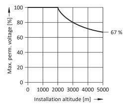
Fig. 27: Derating the voltage depending on installation elevation
