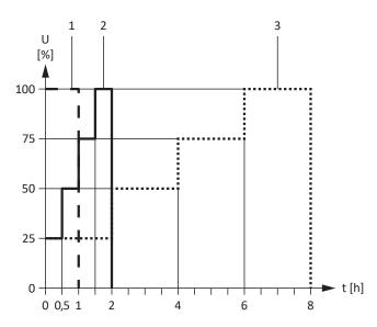
Fig. 31: Voltage levels dependent on storage time
