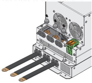
5. Use the screw and washer assemblies (M6, 4.5 Nm, 40 Lb.inch) to fasten the flex cable D+ to D+ of terminal X22, flex cable D- to D- and flex cable of the grounding conductor to ...
