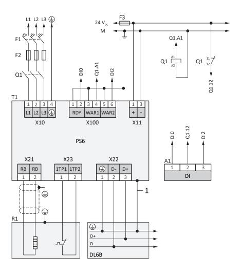
Fig. 98: UL-compliant wiring example with a PS6A44 supply module
