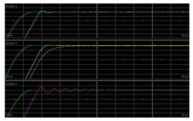
Fig. 64: Scope – Proportional coefficient of the velocity controller (C31), overshooting
