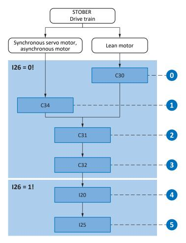
Fig. 58: Schematic sequence of optimization based on relevant parameters
