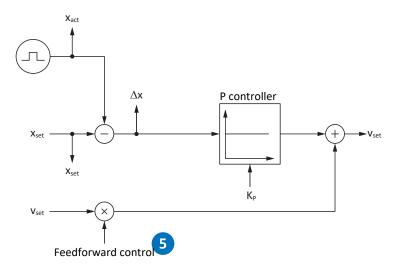
Fig. 68: Position controller – Feedforward control of the velocity controller
