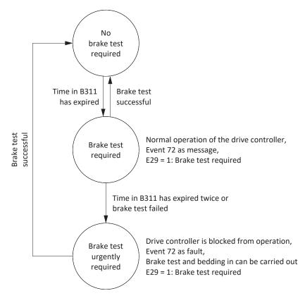
Fig. 76: State machine of brake management
