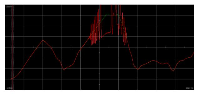
Fig. 69: Scope – Motor reaches saturation without tracking (B59)
