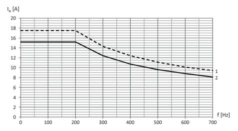
Fig. 23: Derating the nominal current depending on the clock frequency, TEP3820-0CS41
