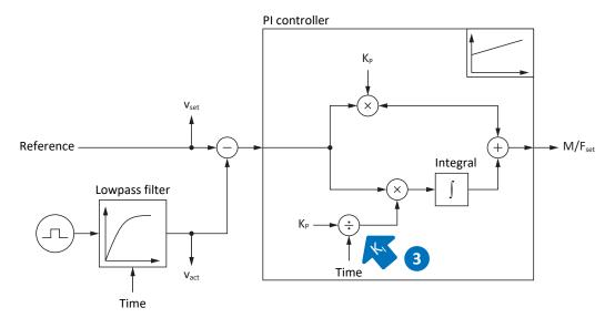
Fig. 65: Velocity controller – Integral coefficient
