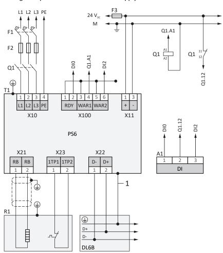
Fig. 97: UL-compliant wiring example with a PS6A24 or PS6A34 supply module  $\,$
