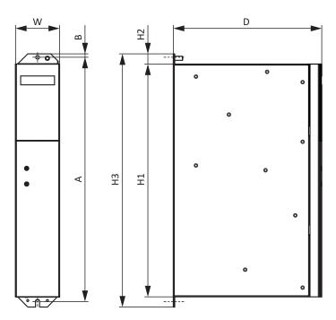
Fig. 7: PS6A24, PS6A34 dimensional drawing
