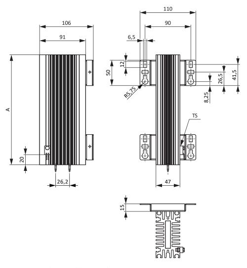
Fig. 14: KWADQU dimensional drawing with MWS310L
