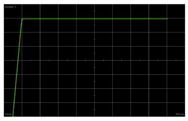
Fig. 63: Scope – Proportional coefficient of the velocity controller (C31), optimized value
