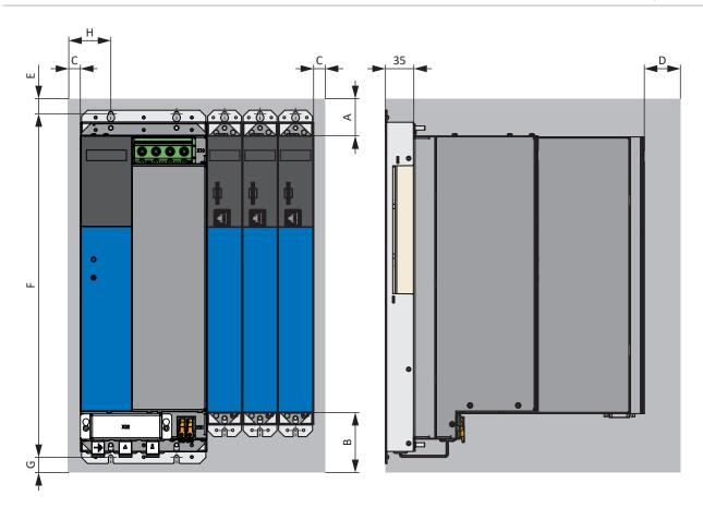
Fig. 34: Minimum clearances for drive controllers in combination with a PS6A44 supply module
