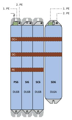
Fig. 28: Grounding concept in mixed operation with powered PS6 supply module
