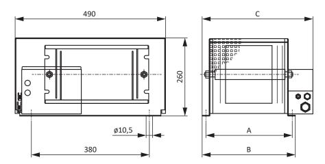
Fig. 16: FGFKQU dimensional drawing
