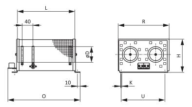
Fig. 15: FZZMQU dimensional drawing
