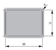
Fig. 39: FZZMQU drilling diagram
