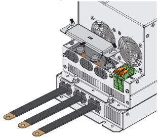
4. Unscrew the 3 screw and washer assemblies on terminal X22.
