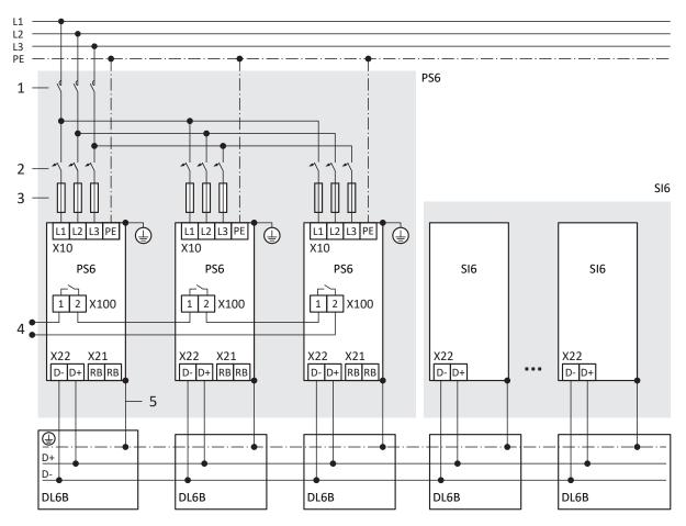
Fig. 96: Wiring example with PS6A24 or PS6A34 supply modules connected in parallel
