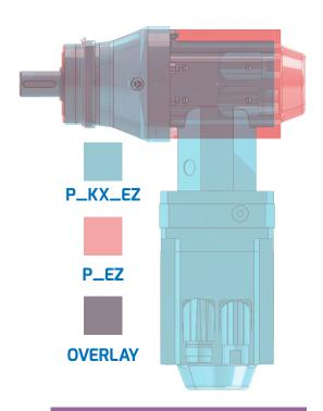
A P\_EZ inline solution overlaid with the same size P\_KX\_EZ solution for size comparison.
