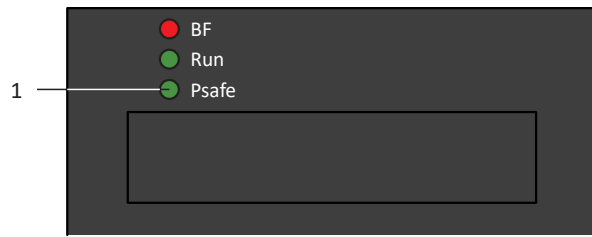
Fig. 7: LED for the PROFIsafe state
