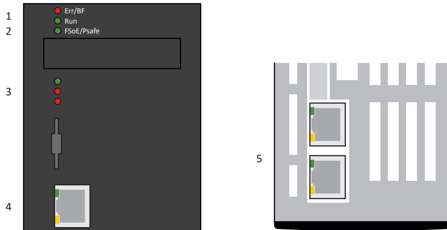
Fig. 61: Positions of the diagnostic LEDs on the front and top of the drive controller
