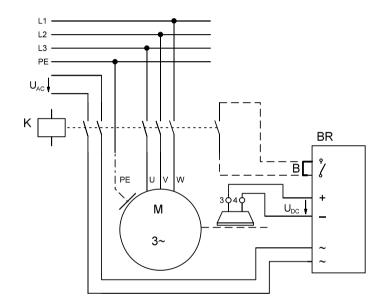
3.3.2.2 Rectifier with power supply from the motor with star configuration
