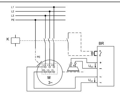
3.3.2.3 Rectifier with power supply from the motor terminals (delta configuration)
