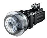
PHQ(A) Planetary Geared Motor PHQ acceleration torque: 84 - 22000 Nm PHQA acceleration torque: 84 - 10000 Nm PHQ backlash:  $\leq 3$  arcmin PHQA backlash:  $\leq 1 - 1.5$  arcmin The ultimate quattro servo drive
