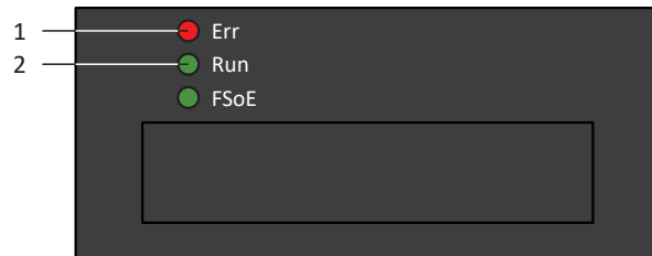
Fig. 5: LEDs for the EtherCAT state
