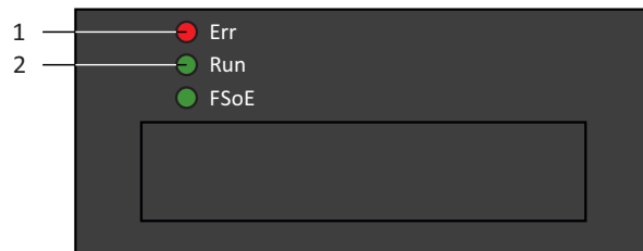
Fig. 3: LEDs for the EtherCAT state
