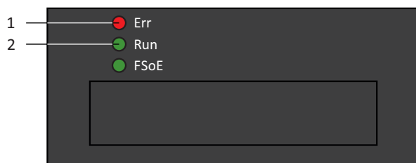
Fig. 3: LEDs for the EtherCAT state
