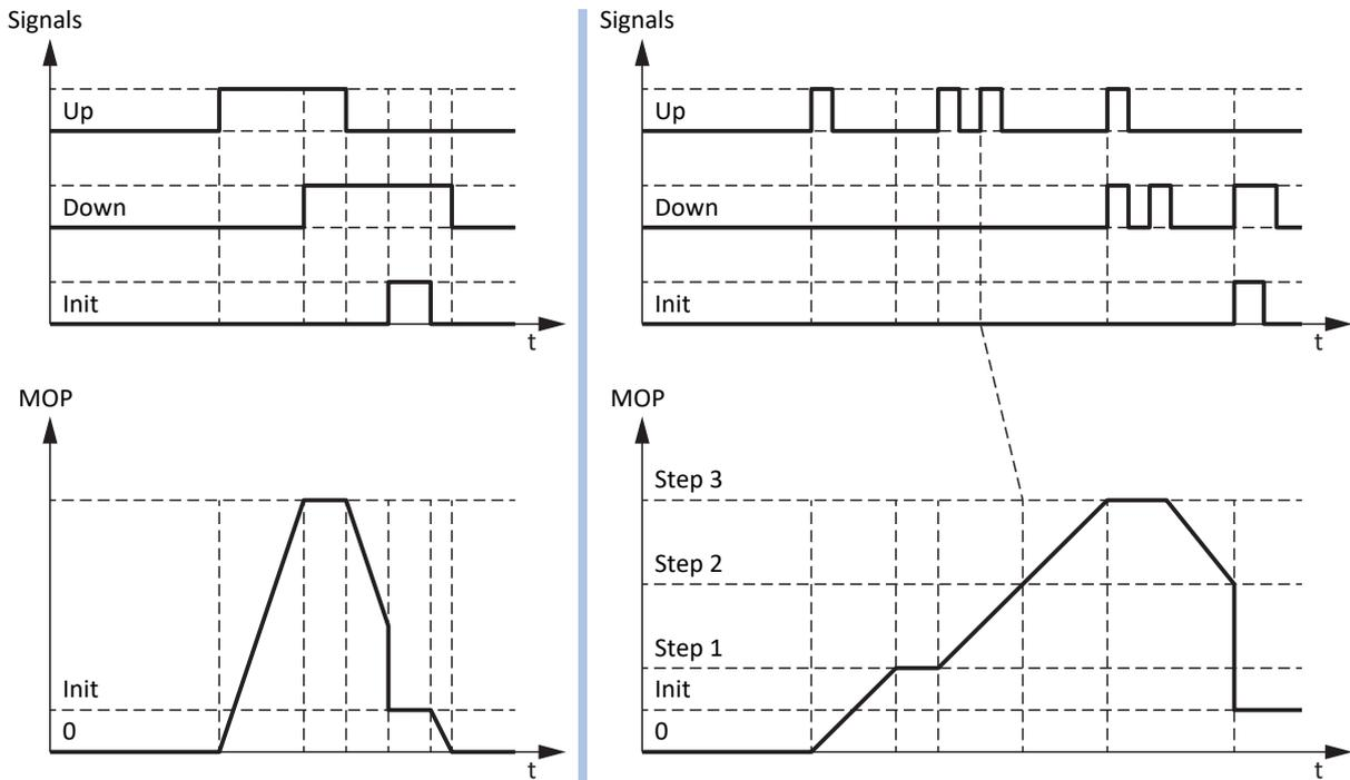
Fig. 7: Motor potentiometer: Linear and stepwise calculation
