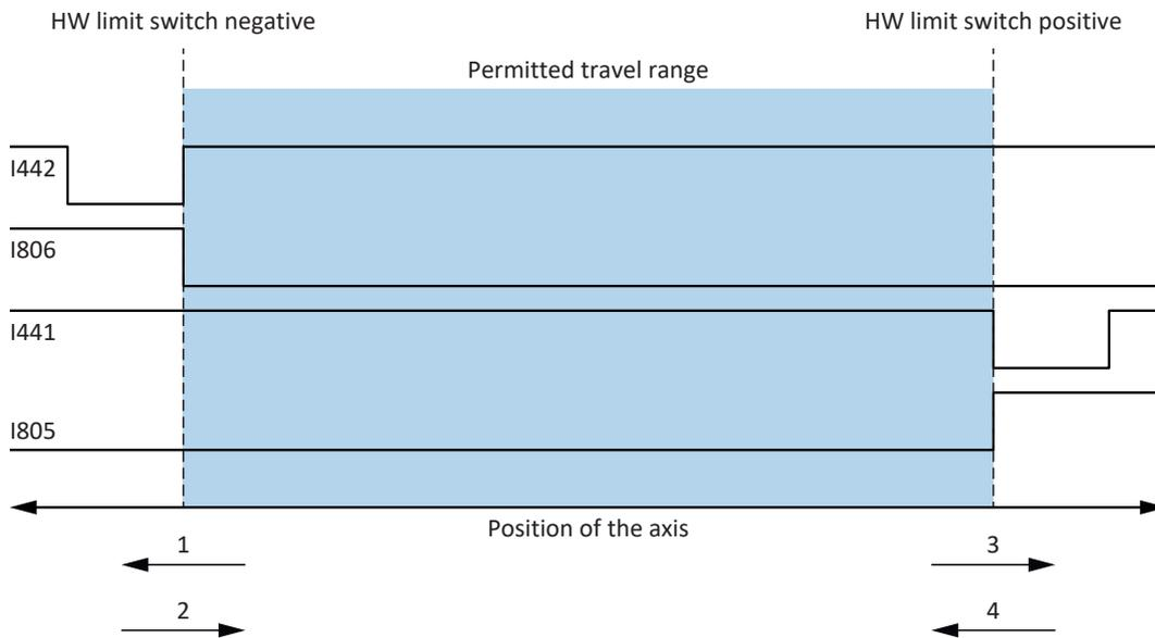
Fig. 17: Hardware limit switch: Limit switch memory
