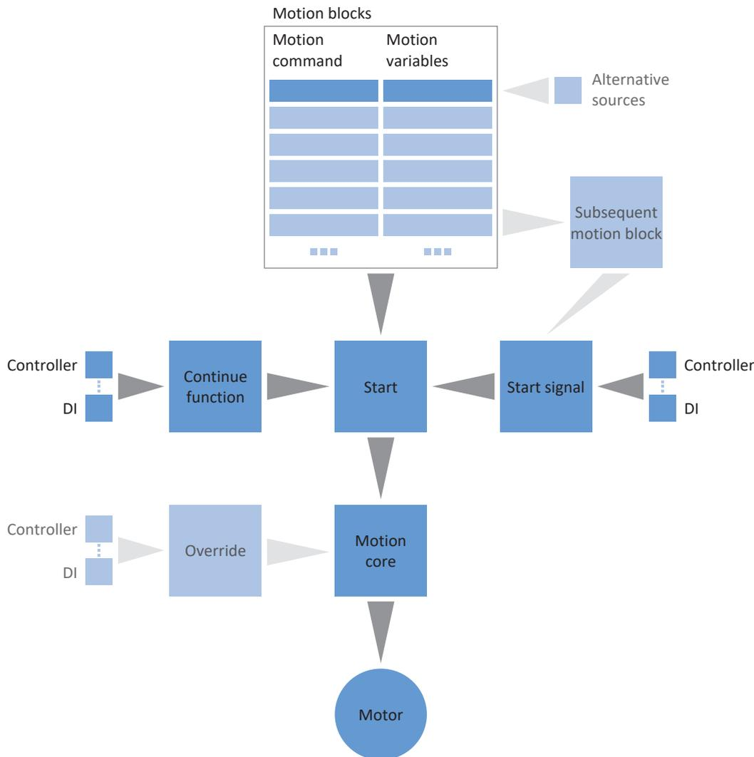
Fig. 3: Motion block operating mode: Signal flows
