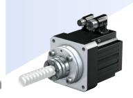
EZS Synchronous Servo Motor for Screw Drives Direct drive of the threaded spindle motor. Shaft as a blind hole hollow shaft. Axial forces (convection cooling): 760 – 31271 N For high axial forces
