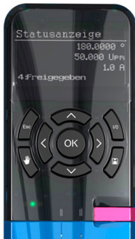
Fig. 24: Operating unit of the SD6 drive controller
