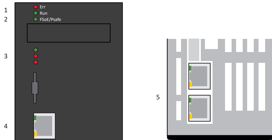
Fig. 59: Positions of the diagnostic LEDs on the front and top of the drive controller
