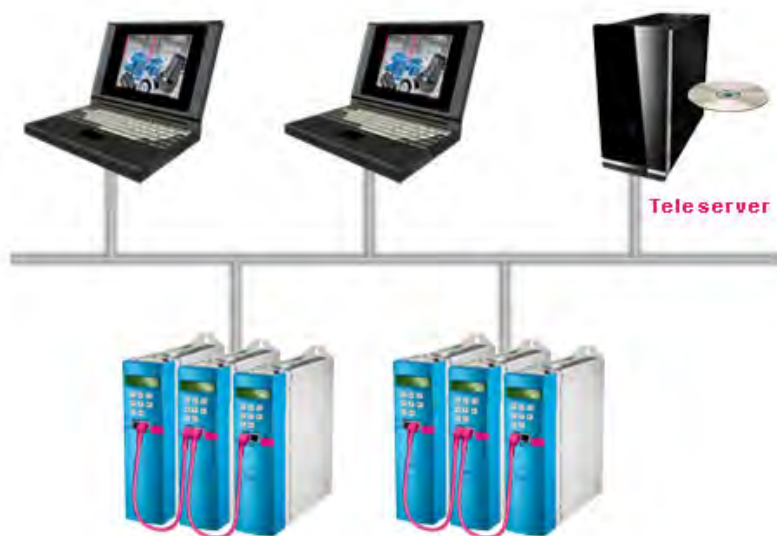
Fig. 11-19: Remote maintenance via the Teleserver
