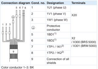
Color conductor 5-8: BK, for 1 mm<sup>2</sup> cross-section: WS
