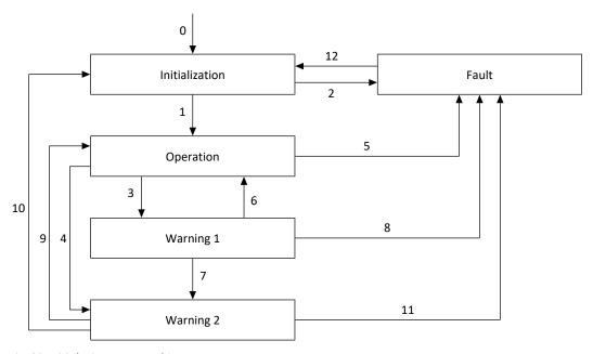
Fig. 82: PS6 device state machine
