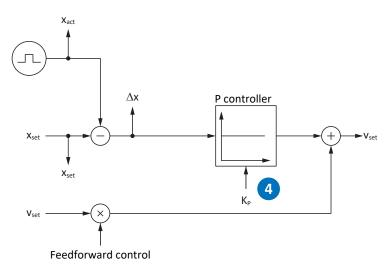
Fig. 68: Position controller – Proportional coefficient
