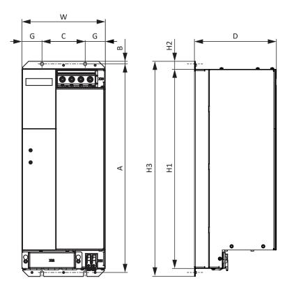
Fig. 8: PS6A44 dimensional drawing
