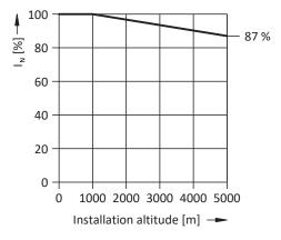
Fig. 26: Derating the nominal current depending on installation elevation
