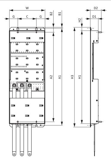
Fig. 12: DL6B22 dimensional drawing
