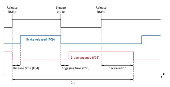
Fig. 76: Minimum time between two release processes for the brake
