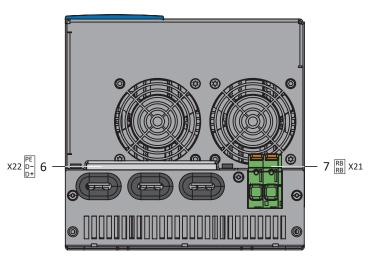
Fig. 48: PS6A44 connection overview, bottom of device
