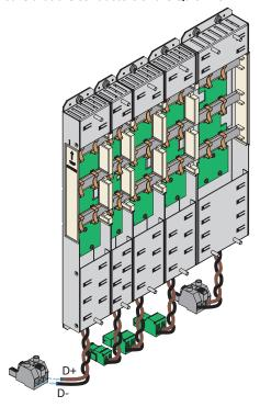
2. Place the drive controller or supply module on the bottom threaded bolt(s) of the Quick DC-Link module and properly align the device vertically with the bottom and top threaded bolts.
