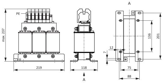
Fig. 17: Power choke dimensional drawing
