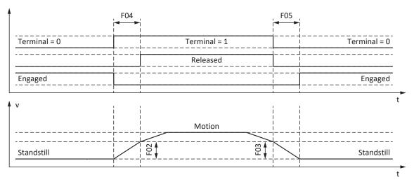
Fig. 72: Brake control for control mode B20 = 0: ASM - V/f-control or 1: ASM - V/f-slip compensated
