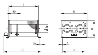
Fig. 15: FZZMQU dimensional drawing
