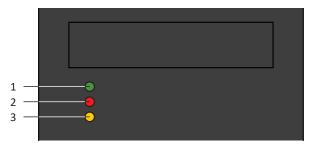
Fig. 81: Diagnostic LEDs on the front of the PS6 device
