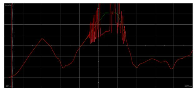
Fig. 70: Scope – Motor reaches saturation without tracking (B59)
