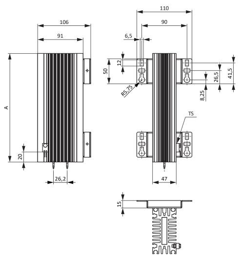
Fig. 14: KWADQU dimensional drawing with MWS310L
