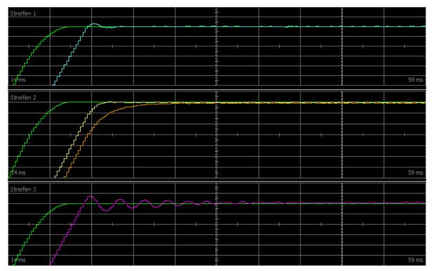
Fig. 65: Scope – Proportional coefficient of the velocity controller (C31), overshooting
