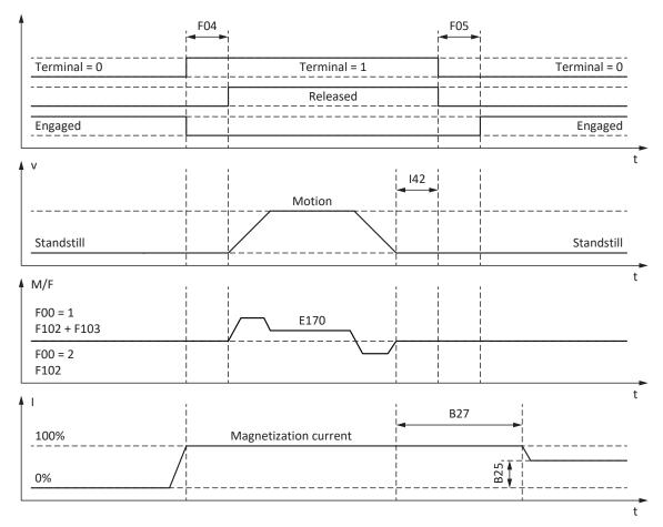
Fig. 73: Brake control for control mode B20 = 2: ASM - vector control
