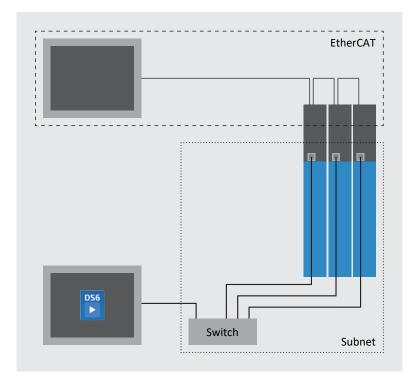
Fig. 94: Multi-axis scope: network structure
