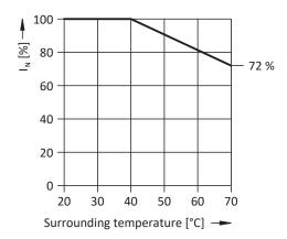
Fig. 25: Derating the nominal current based on surrounding temperature
