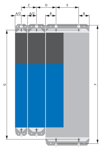
Fig. 36: DL6B22 drilling diagram
