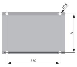
Fig. 40: FGFKQU drilling diagram
