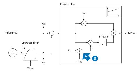
Fig. 66: Velocity controller – Integral coefficient
