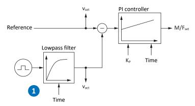
Fig. 60: Velocity controller – Filters for the actual velocity
