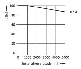
Fig. 20: Derating the nominal current depending on installation elevation
