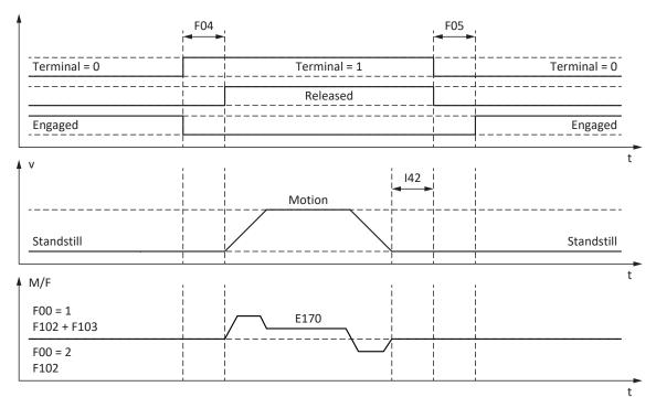
Fig. 75: Brake control for control mode B20 = 32: LM - sensorless vector control, 48: SSM-vector control incremental encoder, 64: SSM - vector control or 70: SLM - vector control
