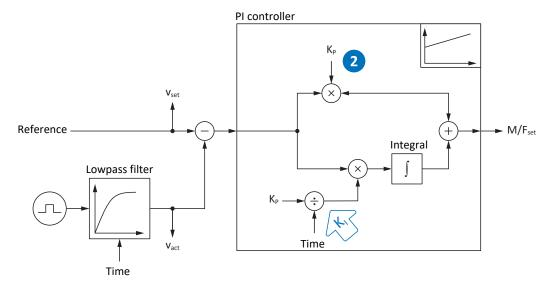
Fig. 61: Velocity controller – Proportional coefficient
