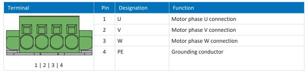
Tab. 148: X20A connection description, sizes 2 (double-axis controllers) and 3
