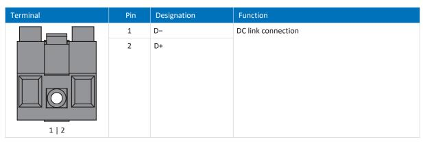
Tab. 152: X22 connection description, sizes 2 (double-axis controllers) and 3
