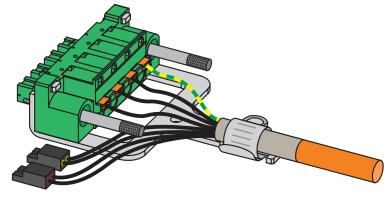
3. Attach terminals X20A and X2A and tighten the screws of X20A.
