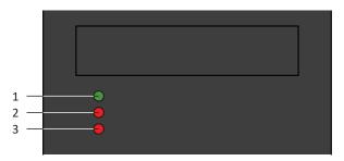
Fig. 88: LEDs for the state of the drive controller
