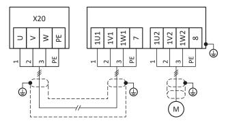
Fig. 54: TEP output choke connection example
