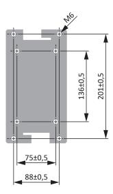
Fig. 41: Power choke drilling diagram
