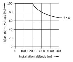
Fig. 21: Derating the voltage depending on installation elevation
