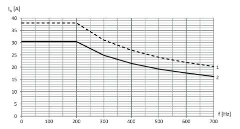
Fig. 24: Derating the nominal current depending on the clock frequency, TEP4020-0RS41
