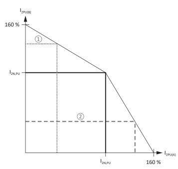
Fig. 9: Asymmetric load on double-axis controllers
