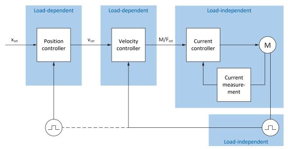
Fig. 58: Structure of the control cascade
