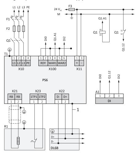
Fig. 97: UL-compliant wiring example with a PS6A24 or PS6A34 supply module
