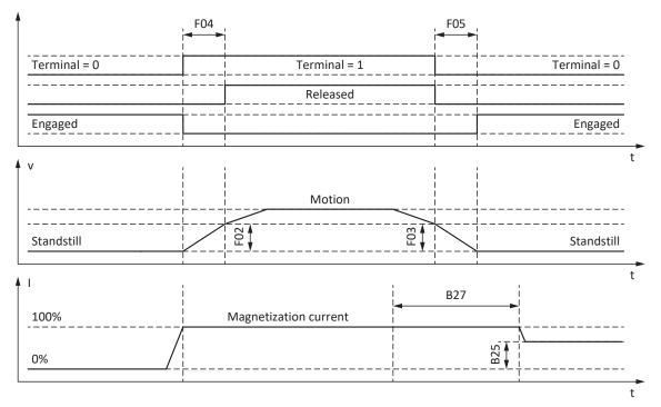
Fig. 74: Brake control for control mode B20 = 3: ASM - sensorless vector control
