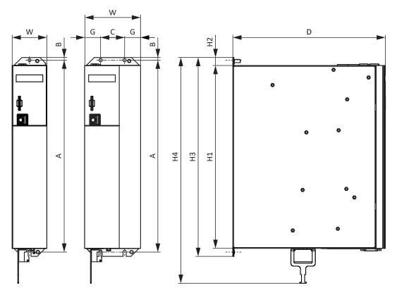
Fig. 10: SI6 dimensional drawing
