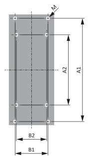
Fig. 42: TEP drilling diagram
