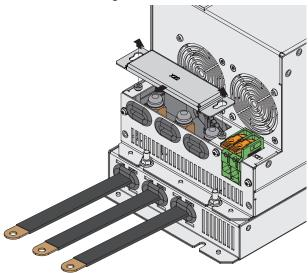
4. Unscrew the 3 screw and washer assemblies on terminal X22.
