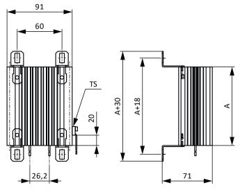
Fig. 13: KWADQU dimensional drawing with MWS306L
