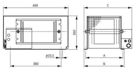
Fig. 16: FGFKQU dimensional drawing
