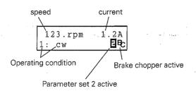
All possible operating conditions are listed on page 24. When the character  $\blacksquare$  lights up, the inverter is operating with parameter set no. 2. If parameter set 1 is active (default setting) there is no special indication in the display. If the brake chopper is active, the  $B_{\mathbb{C}}$  character will appear in the display.
