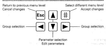
To set the parameters press the # key (Enter). The menu consists of 6 groups, which are identified by the letters A...F. Use the serious keys to select a group, then press the # key to access the parameters of the group selected.
