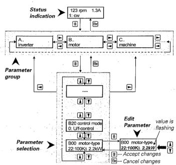
After power-up the inverter will only display the most important parameters required for commissioning. If your drive application requires more complex-parameter settings, you may activate the extended menu level by setting A10 = 1.
