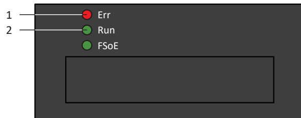
Fig. 60: LEDs for the EtherCAT state
