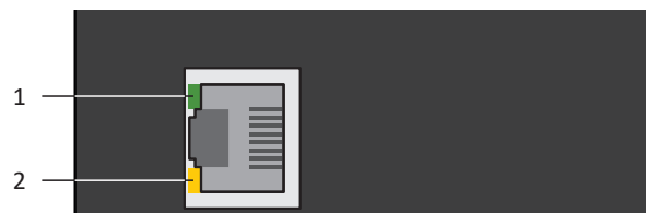
Fig. 65: LEDs for the state of the service network connection
