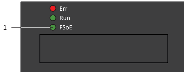
Fig. 61: LED for the FSoE state
