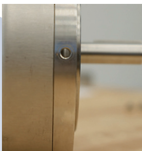
Weep holes on typical NEMA Motor
