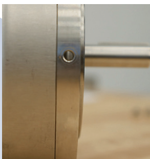
Weep holes on typical NEMA Motor
