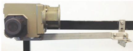
A reducer with a typical torque arm.
