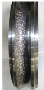
Examples of an inner and outer bearing race damage from excessive axial loading.
