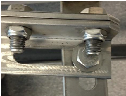
A reducer with a typical torque arm.
