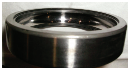
Above and left: outer and inner bearing race with radial load damage. Below: output bearing damage due to radial/overhung loads.
